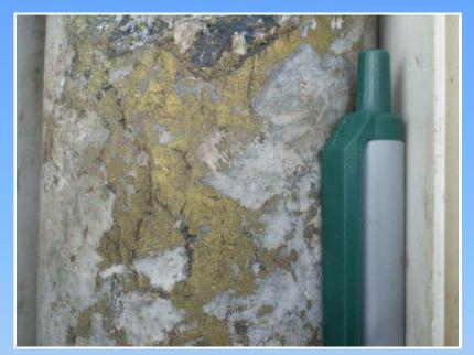
NAK2-003 drillhole site with visible malachite stains on outcrops (left) and Drillcore sample at 78 m depth (above)
