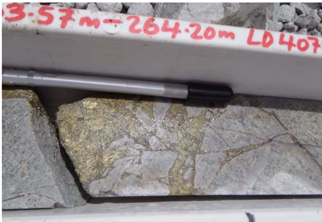
PHOTO 1: High Grade Veining in Drillcore BWNBDD0014 at 264.2 metres Depth Assaying 4.2% Copper over 1 Metre
