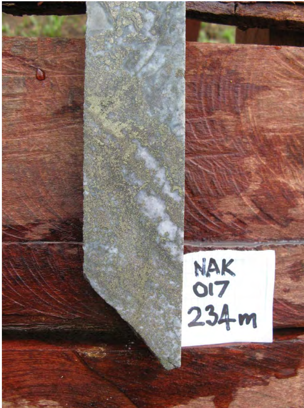
Photo 2: Copper and Iron Sulphides in Drill Core (NAK17A)
