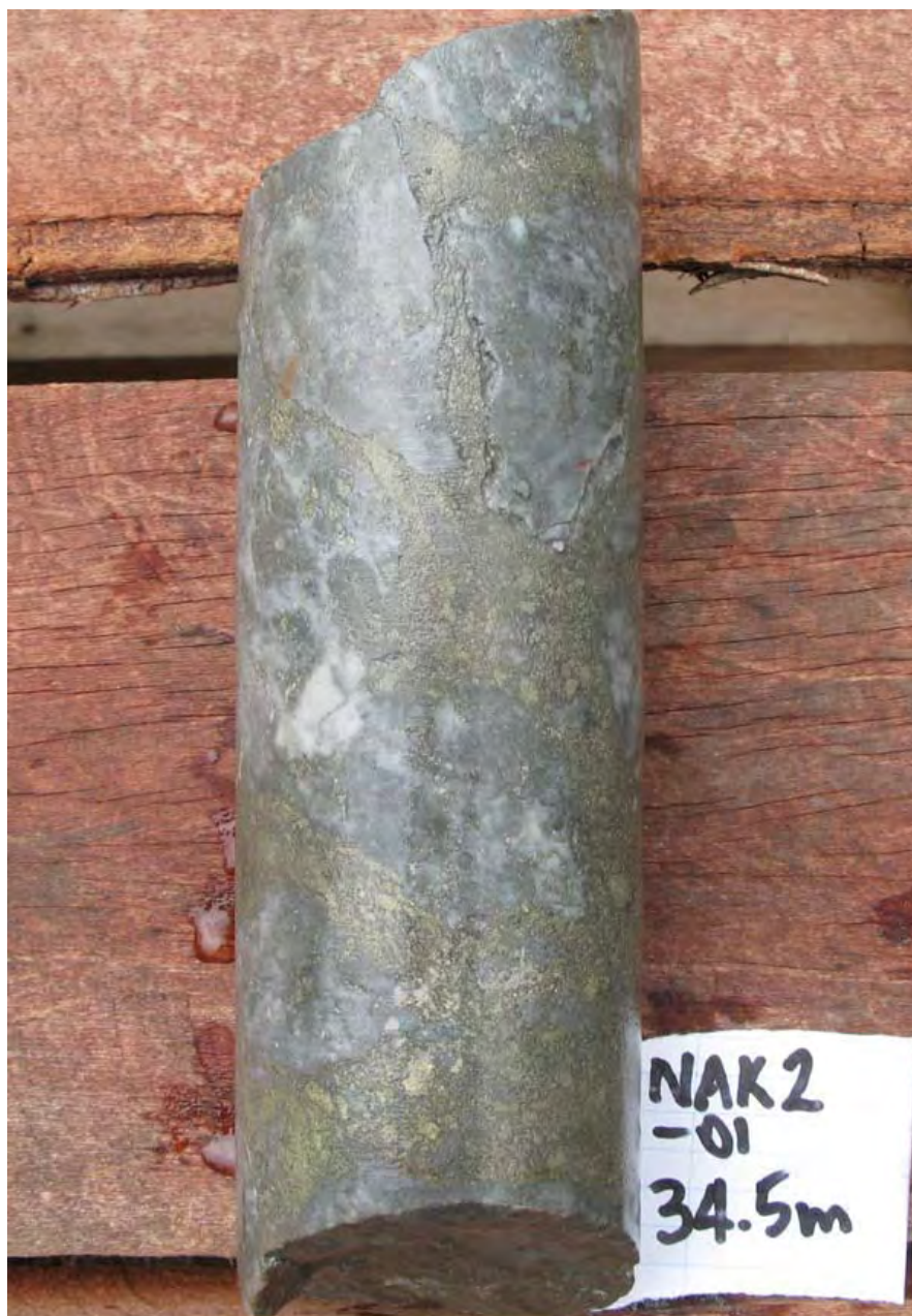
Photo 3: Sulphide Rich Matrix Fill Mineralisation in Silica Breccia (NAK02-001)
